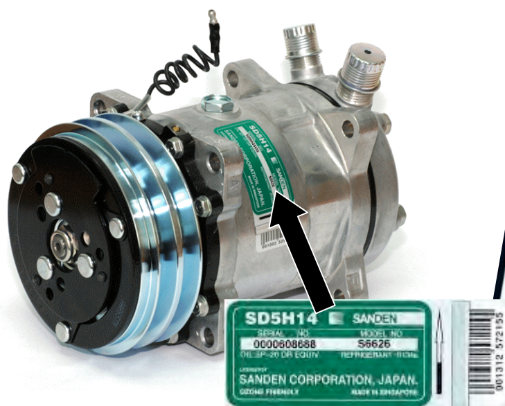
Sanden label with unique barcode and tag
