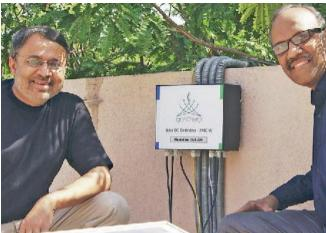
Solar installations face large energy losses due to shadows falling on panels (buildings, poles, clouds), dust and bird droppings, high temperatures, degradation, wear and tear. The Optimizer, a product created by igrenEnergi helps increase the harvest of solar energy from solar installations by 10-20% or even more.
